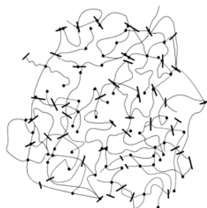
Figure 2. Structural model of the 3-D network with both magnetic particles (dots) and ATP nanorods (lines) as cross-linkers.
